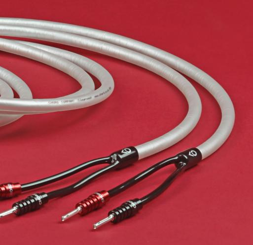
With this budget and affordable new cable Chord has made improvements. The Clearway X has a new and more expensive XLPE (cross-linked polyethylene) insulation, replacing the original's FEP (fluorinated ethylene propylene) that Chord used because it had the "same electrical characteristics" as the PTFE found in costlier cables. The two conductors, built from multiple strands of highpurity oxygen-free copper are arranged in a twisted-pair configuration; this, say Chord, will "reduce interference"
