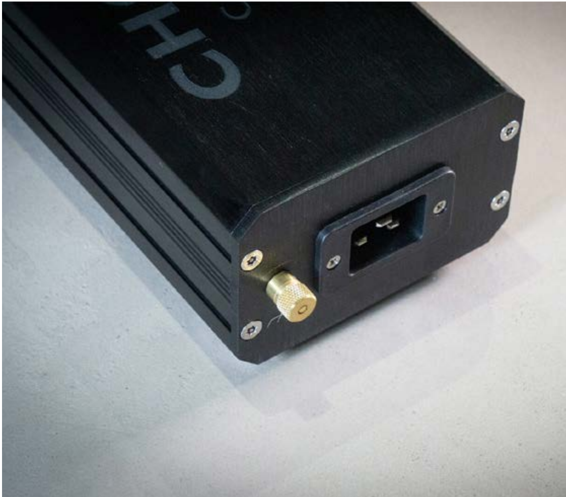
Mains inlet resides on one end, alongside a handy heavy-duty earthing clamp
